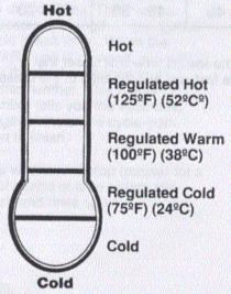
The regulated wash temperatures are obtained by turning both the hot and cold water valves on initially. During the fill, the hot or cold water valve will turn off, leaving only one valve on until the end of the fill. Therefore, the water entering the tub may be only hot or cold. This is normal operation.
